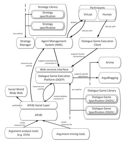
Fig. 4. The DGEP application architecture.
